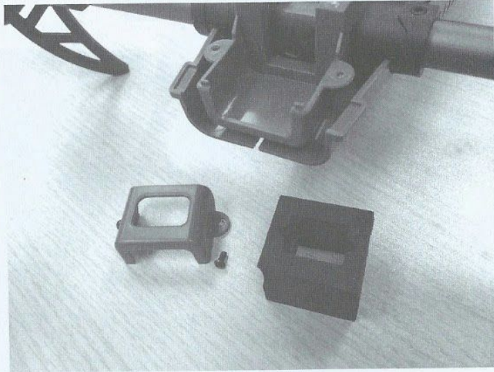
FPV camera tray on the front and video transmitter slot at the back allows players to install devices upon their choices
