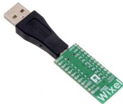
Together, the USB Adapter A to Mini-B and a Pololu Wixel wireless module can make a compact USB dongle.
