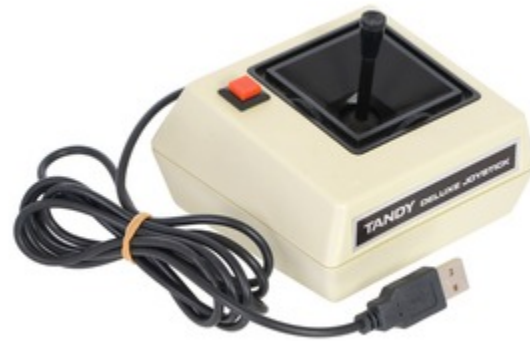
This converted Tandy Deluxe Joystick is now usable as a USB Human Interface Device.
