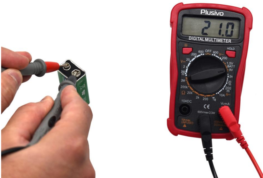
Fig. 7. The measured current in this figure is 21 mA
