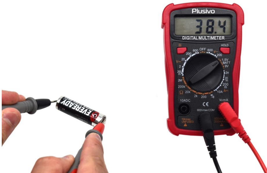
Fig. 6. The measured current in this figure is 38.4 mA
