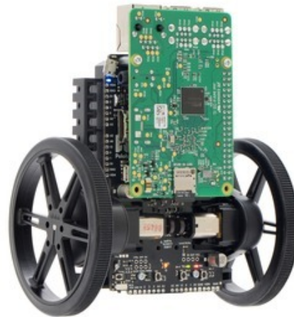
Balboa 32U4 Balancing Robot with 80×10mm wheels and a Raspberry Pi 3 Model B.
