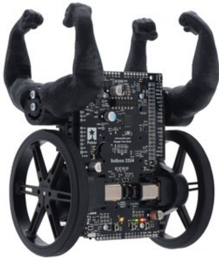
Balboa 32U4 Balancing Robot with 80×10mm wheels and 3D-printed arms.
