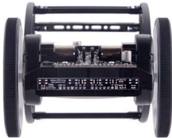
Center-aligned mounting option for the 5-Channel reflectance sensor array for Balboa.
