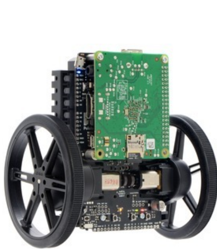
Balboa 32U4 Balancing Robot with 80×10mm wheels and a Raspberry Pi 1 Model A+.
