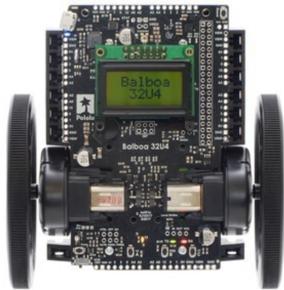
Balboa 32U4 Balancing Robot with 80×10mm wheels and LCD.
