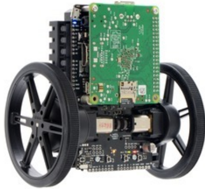
Balboa 32U4 Balancing Robot with 80×10mm wheels and a Raspberry Pi 1 Model A+.
