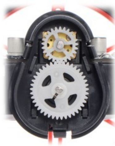
A look inside the external gearbox on the Balboa 32U4 Balancing Robot.
