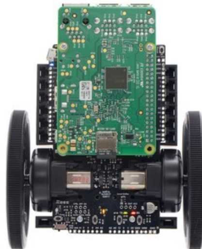
Balboa 32U4 Balancing Robot with 80×10mm wheels and a Raspberry Pi 3 Model B.
