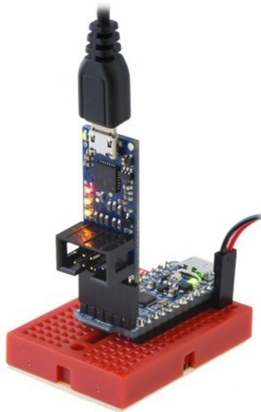
The Pololu USB AVR Programmer v2 (top) connected to an Adafruit Pro Trinket for programming.
