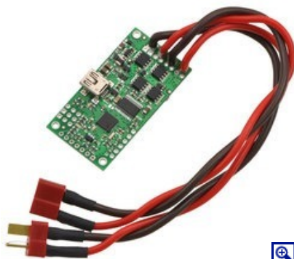
Simple High-Power Motor Controller 18v15 or 24v12, partial kit with custom power and motor connectors (NOT included).
