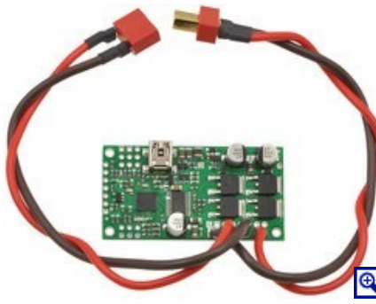
Simple High-Power Motor Controller 18v25 or 24v23 with custom power and motor connectors (NOT included).
